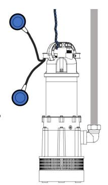
All single phase models have automatic reset thermal overload protection built in. This thermal overload will switch the motor off in an overload/overtemperature situation and will automatically reset when the motor has cooled down.
